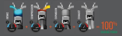
The absorbed power during compression is returned to the piston by the rebound of the expansion cycle.
